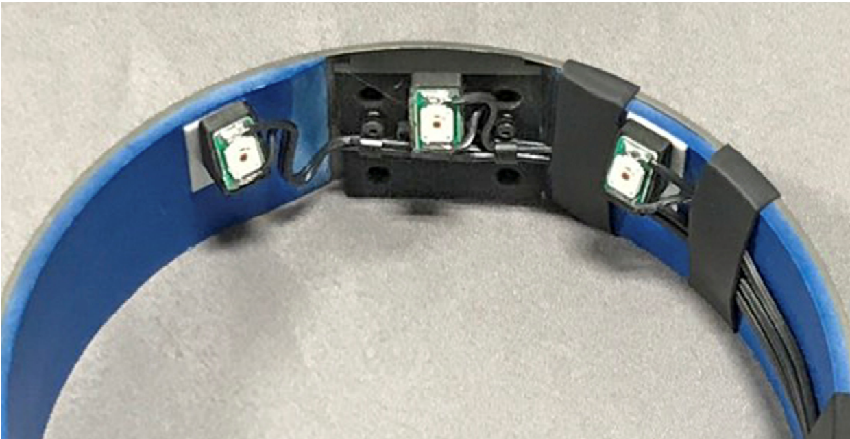
Figure 21. Alternative mounting of rearward and forward LEDs
