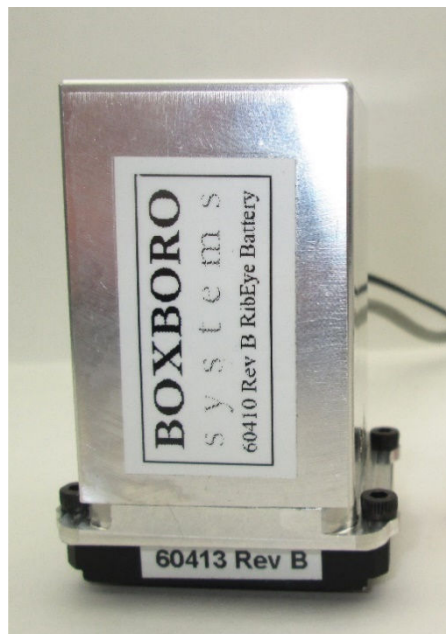
Figure 6. Battery pack and the adaptor for mounting the battery pack at the shoulder rib
